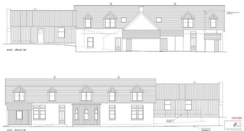
Fig. 3 : Originally proposed western and eastern elevations, with the introduction of a series of new dormer windows in the roof space
